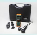
Extech's compact UV Light Meter includes two types of probes: one to measure UVA (long wave 365nm) and the other to measure UVC (short wave 254nm) light sources up to 20mW/cm<sup>2</sup>. The UV800 date/time stamps and stores files onto a 2GB SD card in MS Excel<sup>®</sup> format to make transferring, storing, and analyzing the data on your PC easier. The unit also has a Type K/J thermocouple input to capture temperature readings (probes not included).
